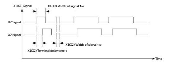
Figure 6-14 X1/X2 terminals delay
